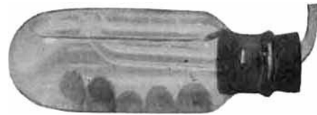
Fig. 2.—Tablets with New Enteric Coating after Ten Hours in Artificial Gastric Fluid. No Evidence of Disintegration Visible.
