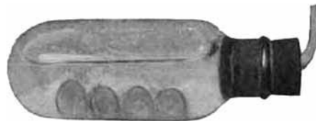
Fig. 3.—The Same Tablets as in Fig. 2, Thirty Minutes after Being Placed in Artificial Intestinal Fluid. Disintegration Is Taking Place.
